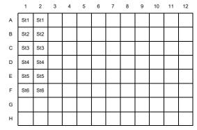
Example plate layout (example for a 6 point standard curve)
